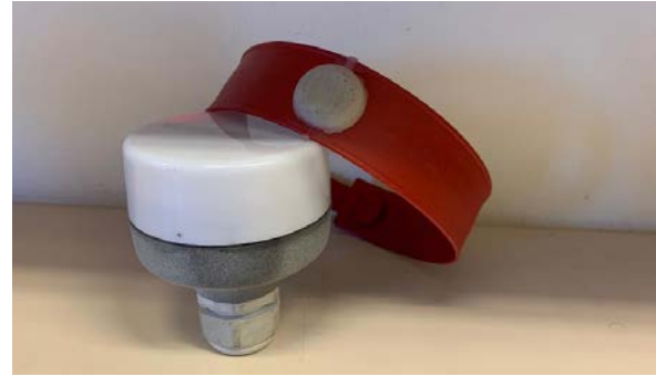
Figure 2. The 2019 generation of the flashlight receiver (left) and the transmitter integrated in a reindeer collar (right) (photo: Johannes Karlsson).
