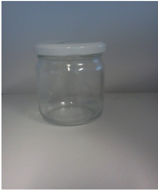
Container used for samples intended for lipids and fatty acids laboratory analyses
