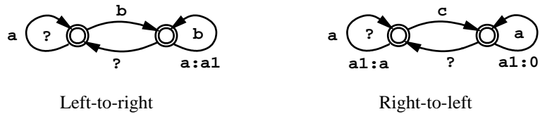
Figure 2.21: Bimachine for [a^+ @ \rightarrow 0 \mid \mid b - c]
