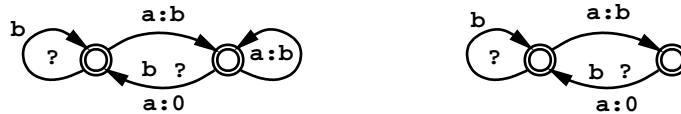
Figure 2.14: The Relation [a \mid a a \rightarrow b] vs. [a \mid a a @\rightarrow b]
