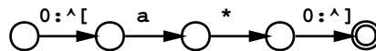
Figure 9.7: A network with a delimited substring that has the format of a regular expression. As far as the network itself is concerned, “a*” is just a concatenation of the two symbols a and * .
